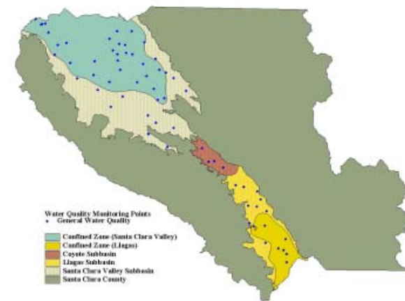
Figure 4-1 Water Quality Monitoring Wells
